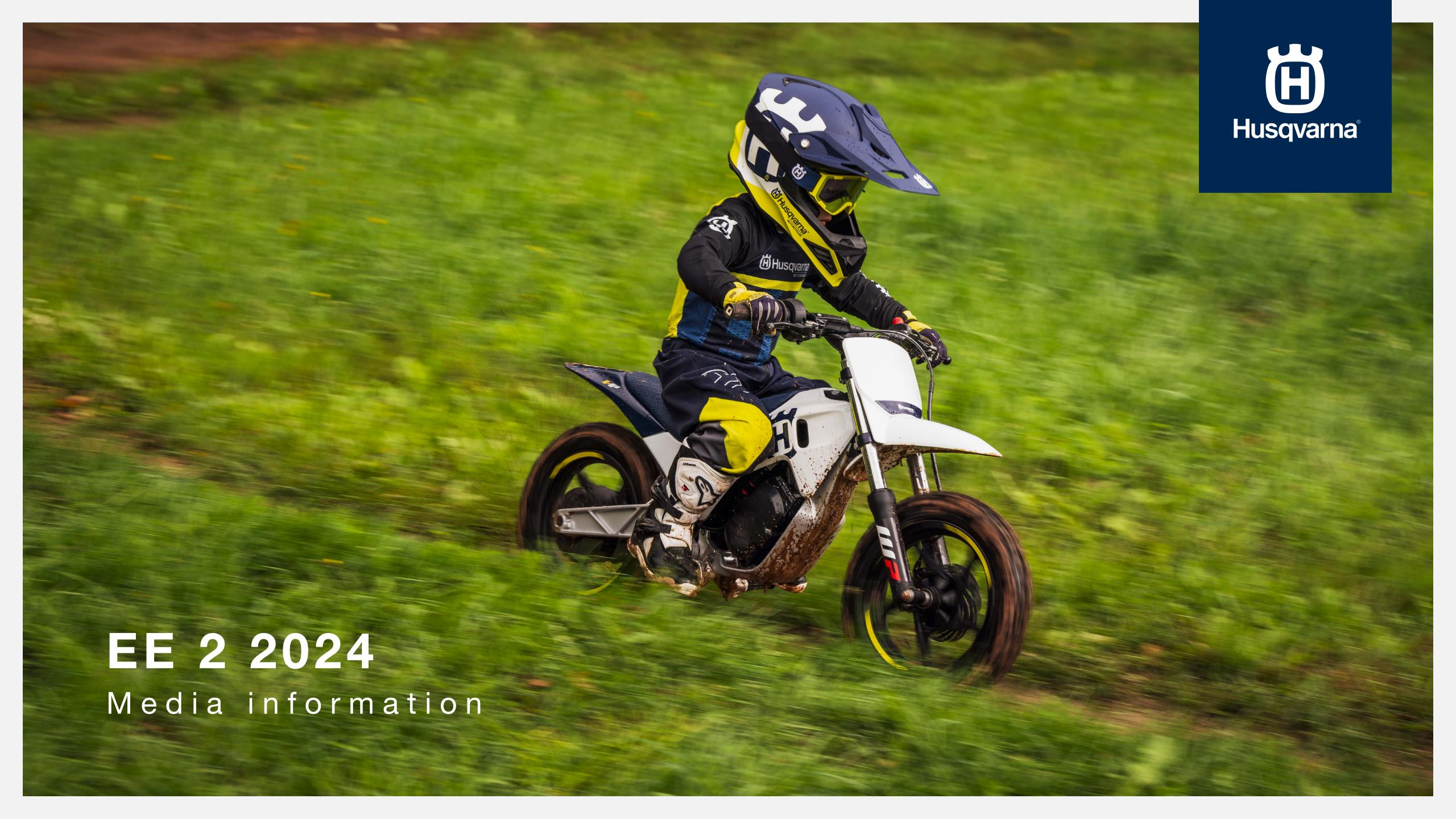
With the electric motor featuring a permanent drive, the need for a clutch or gearbox is eliminated, allowing children to focus on the fundamental skills needed to ride safely – starting, stopping, and cornering. Additional benefits of the electric powered motors are that they are dust and waterproof, they offer near-silent operation, and the fact that they are completely maintenance free.
